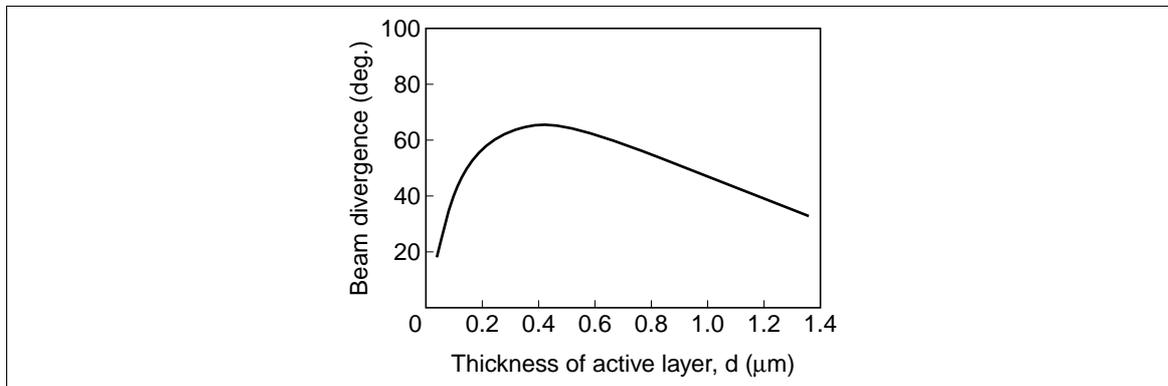
**Figure 2-6 Thickness of Active Layer vs. Beam Divergence**
