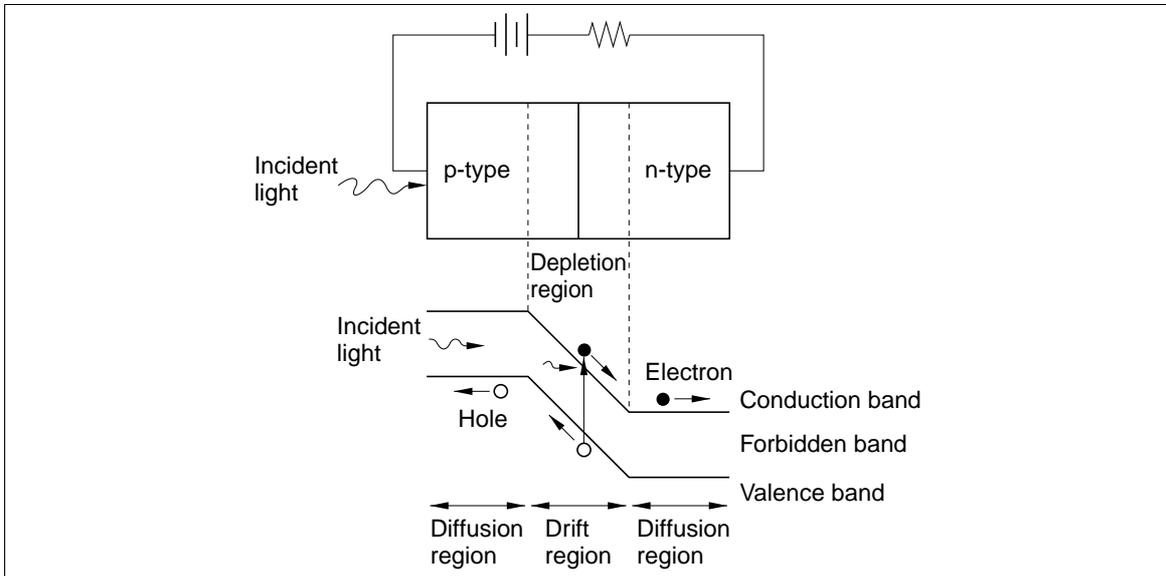
**Figure 1-4 Photo-detection Principles**
