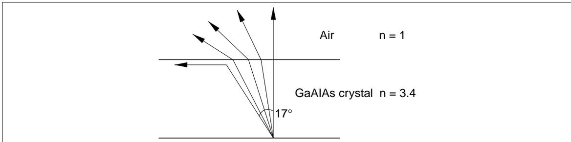
**Figure 2-12 Light Refraction at Boundary Layer**
